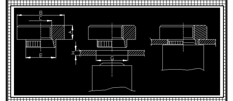
These special nuts are to be used on thin metal supports.
